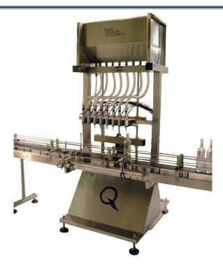
A Gravity, or Pressure Gravity, Filling Machine provides a time-based fill system with individually timed fill heads, making it one of the most accurate and economical fillers for products that are consistent in viscosity. Typical products include water, edible oils, distilled spirits, molten products, corrosive products, and more!
